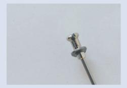
n the theoretical ideal wheel, the nipples are a perfect fit on the spoke ends, and the nipple head leans on the border of a perfectly- shaped hole in the rim, all spokes, all nipples and all spoke holes are identical.
