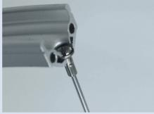
inate friction between its components. For the friction between spoke and nipple, there is basically only one solution: precise machining by the spoke maker. The spoke manufacturer is nearly always the same as the nipple manufacturer, so it is his technology and quality standard to make these parts fit, to indicate the maximum tension and torque. Manufacturers of quality spokes are aware of the imperative character of an absolutely consistent product, and all conform to ISO standards.
