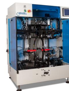
For efficient production predictability is a must. Therefore, AI has made its entry in the production of wheels at Holland Mechanics. Traditionally the wheel truing setting of the spoke tension was based on trial and error. Sensors observed each
