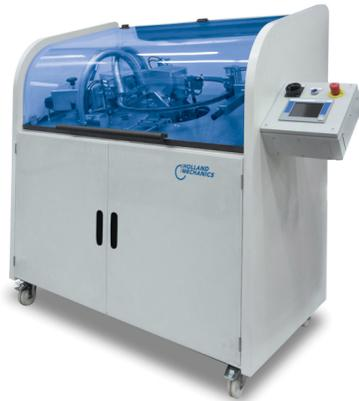
The Holland Mechanics High-end rim drilling station has revolutionized the art of drilling spoke holes into carbon and other high-end rims. With the ability to drill all possible spoke patterns in all angles, these ultra-light carbon bicycle rims are now more customizable than ever before.
