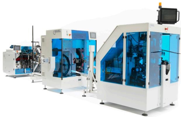
Holland Mechanics gains popularity worldwide with its 4<sup>th</sup> generation high-end wheel assembly line, which integrates all the aspects of wheel building craftsmanship with advanced robotics to produce some of the best wheels on the market. The company has made efforts to develop a state-of-the-art assembly line due to the scarcity of hand wheel builders globally.
